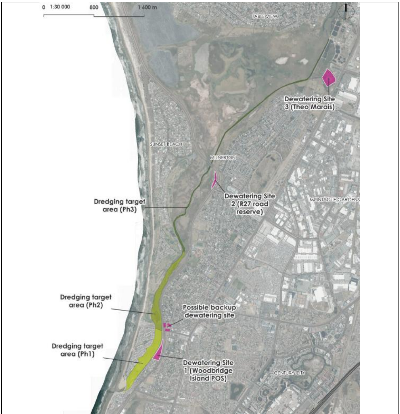
Figure 14: Visual representation (extracted from Figure 5-13 of Rose et al. (2023)) of the three phases initially proposed for dredging within the lagoon and the corresponding dewatering areas.
