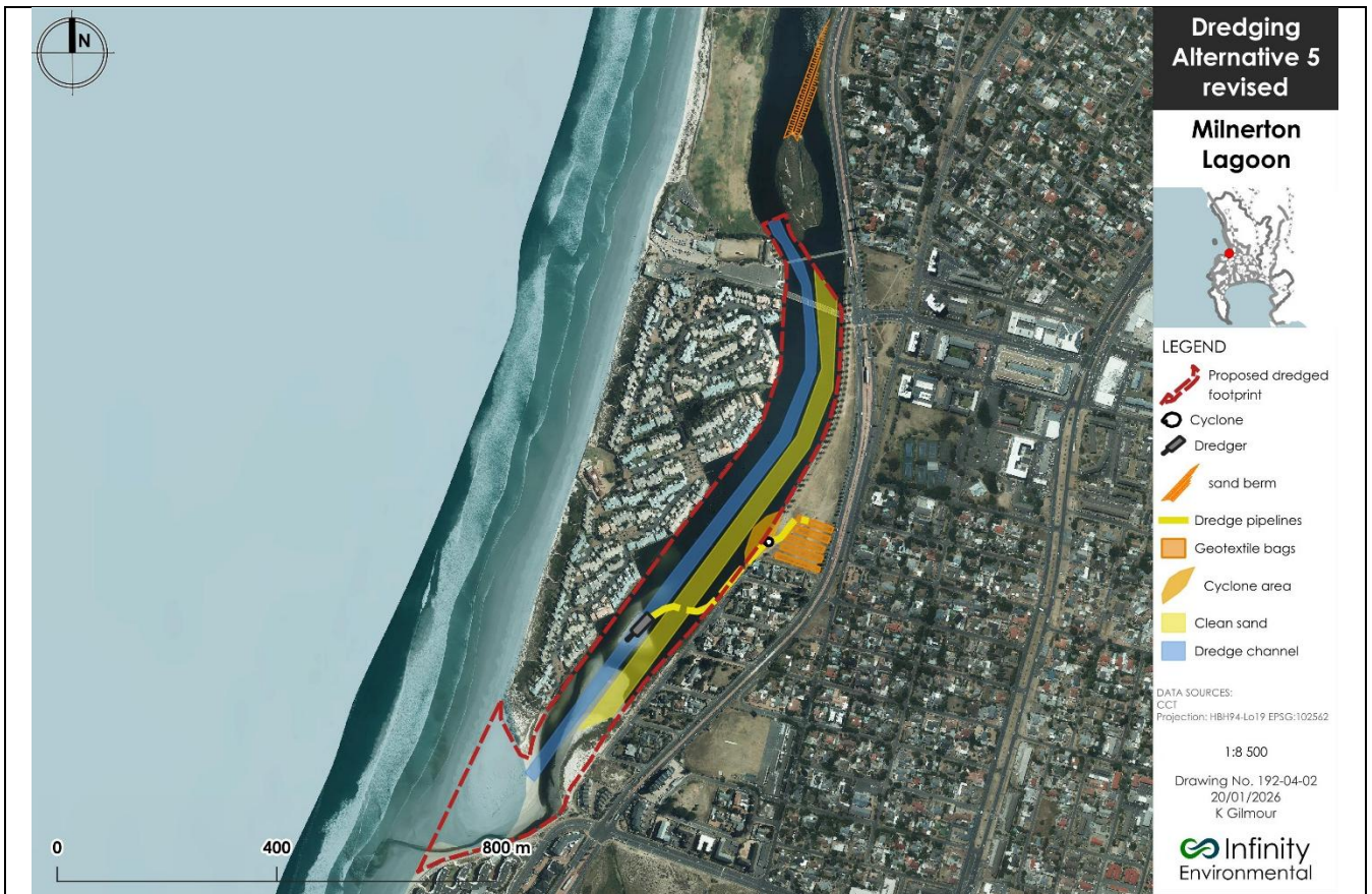
Figure 19: This schematic presents the design and layout Alternative 5 – the proposed dredging with off-site disposal.
