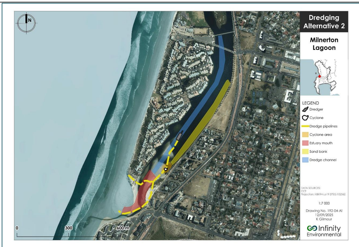
Figure 16: This schematic presents the design and layout Alternative 2 – the proposed dredging with cyclone separation and disposal at lagoon mouth.
